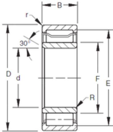
A-5236-WS Bearing 2D drawings and 3D CAD models
